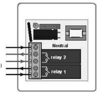
**IMPORTANT:** Halogen, electronic fluorescent and low consumption lamps present a very high consumption (up to 20Amp) at switch-on and switch-off time, rapidly damaging relay contacts. If this type of lamps are being used, Onity recommends to check if the use of a contactor is required.
