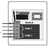
IMPORTANT: Halogen, electronic fluorescent and low consumption lamps present a very high consumption (up to 20Amp) at switch-on and switch-off time, often damaging relay contacts. If this type of lamps are being used, Onity recommends to check if the use of a contactor is needed.
